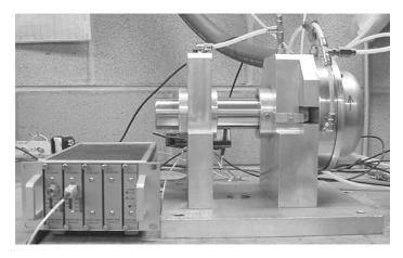
Fig. 10: Journal Bearing Test Rig (R&D Dynamics Corp.)
