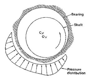
Fig. 1: Principle of an Air Bearing
