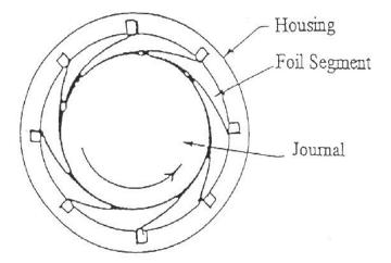
Fig. 3: Multipad Foil Journal Bearing Schematic
