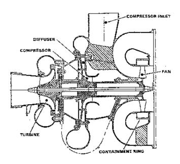
Fig. 17: 767/757 Foil Bearing Air Cycle Machine (Developed by AiResearch)
